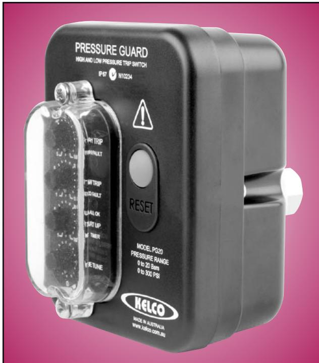
*The Kelco PG20 Pressure Guard is a dedicated pressure operated safety device that can be set to shut down a pump if the system pressure exceeds a preset level or falls below a preset level. It can be set for over pressure protection, under pressure protection or both.*
