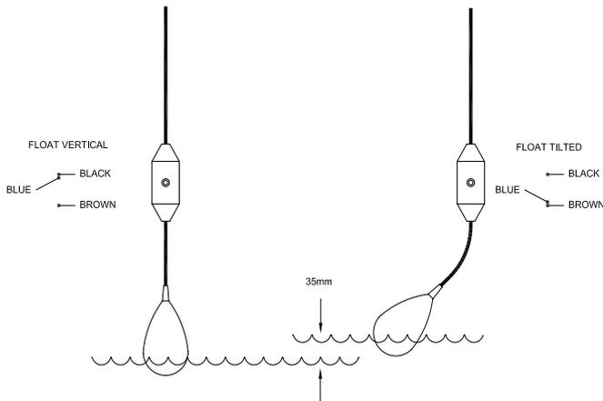
The KU series heavy duty level regulator is rated at 240VAC. However, in the interests of safety the KU series level regulator should only ever be used with control voltages in the range of 12 volts to 24volts AC or DC
