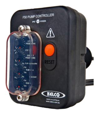
The F50 advanced pump controller is a pump control computer that learns from its environment and adapts itself to the pressure and flow conditions it finds in a pump system. It is able to control a pump within settable pressure limits and yet operate on flow. It gives the user constant pressure at the tap and also protects the pump from running dry.
