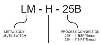
H = STANDARD HEAVY DUTY SWITCH L = LOW VOLTAGE SWITCH WITH GOLD CONTACTS
