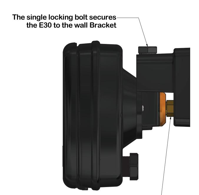
Screw a 1/4 BSP 90 Degree elbow (not supplied) into the process port on the E30. The inlet port on the elbow must be alligned downward to accept a capillary tube adaptor and to stand clear of the wall
