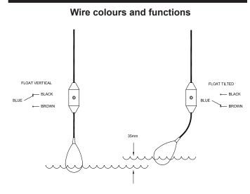
The KU series heavy duty level regulator is rated at 240VAC. However, in the interests of safety the KU series level regulator should only ever be used with control voltages in the range of 12 volts to 24volts AC or DC
