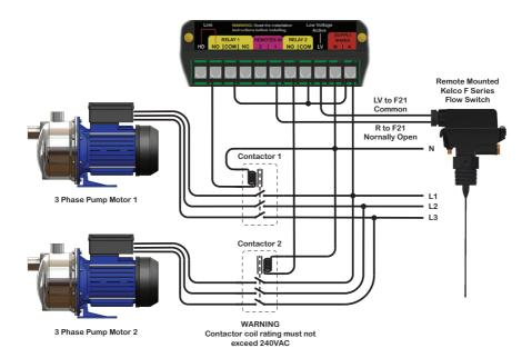
In the diagram above, the F60 MK3 would normally be installed in the discharge pipe of pump 1. The remote flow switch would normally be installed in the discharge pipe of pump 2. The remote flow switch can be a paddle style switch such as the Kelco F Series as depicted or an in line style flow switch such as a Kelco C25-B. The remote flow switch must have voltage free normally open contacts.
