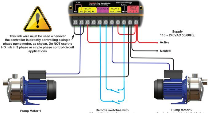
110 ~ 240VAC 50/60Hz Pump Motor 2.4kW Max. when the HD terminal is linked
